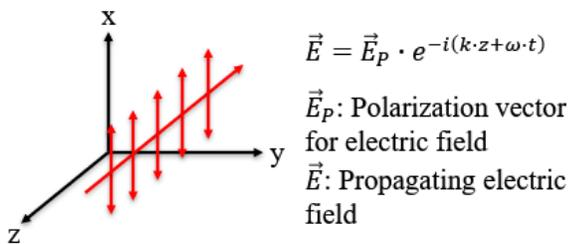
Figure 3. Wave polarized in the x-direction and propagating in the -z-direction
