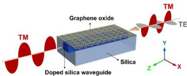
Figure 15. Integrated Waveguide Polarizer Example
