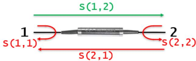
Figure 2. Optical isolator as 2-port Element
