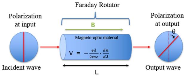
Figure 5. Rotation of Polarization using Faraday Effect
