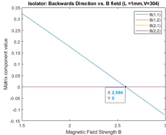
Figure 9. Backward Direction, Polarization from Isolator vs. Magnetic Field Strength
