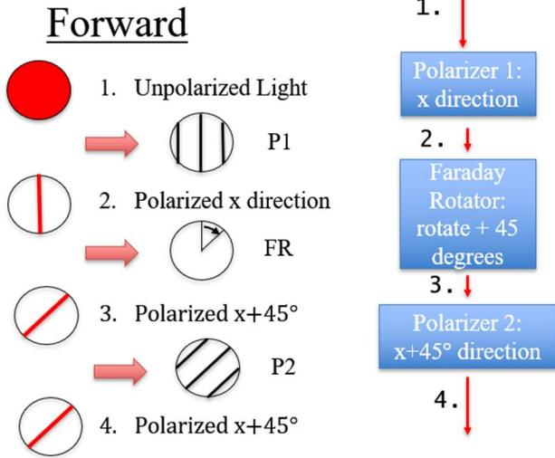
Figure 6. Optical Isolator in Forward Direction
