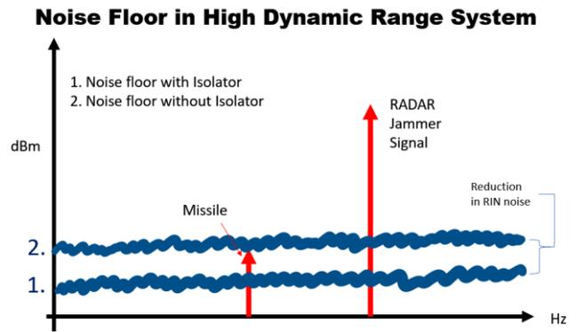
Figure 14. High Dynamic Range Integrated Microwave Photonic System
