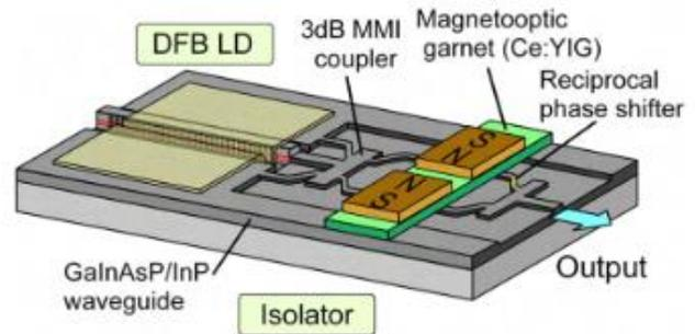
Figure 19. Integrated Isolator Design on InP with DFB Laser
