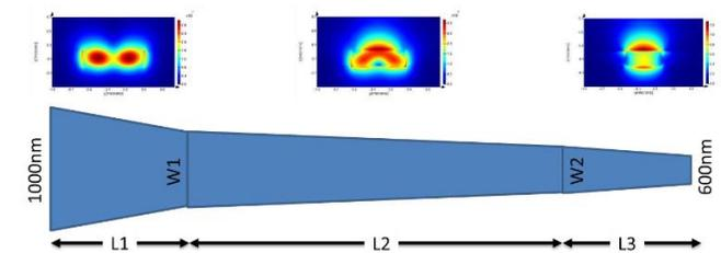
Figure 17. TE1 to TM0 Converter for Integrated Isolators
