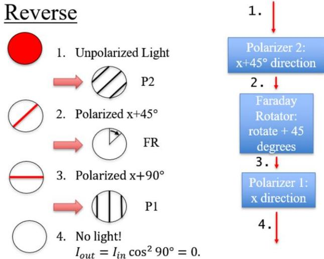
Figure 7. Optical Isolator in Reverse Direction
