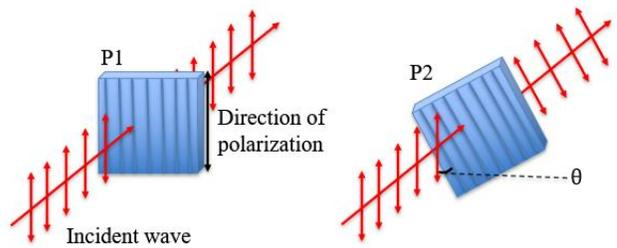
Figure 4. The angle between polarizers and incident waves
