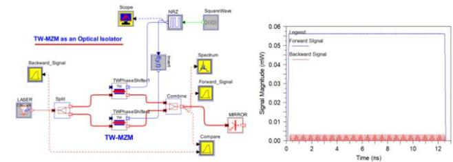
Figure 16. Travelling-Wave MZ Modulator as Isolator
