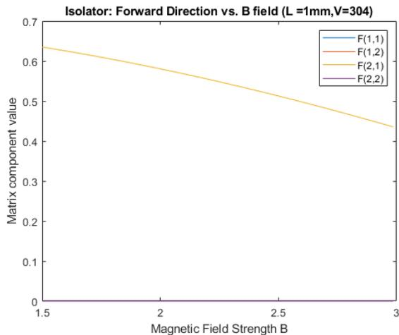
Figure 8. Forward Direction, Polarization from Isolator vs. Magnetic Field Strength
