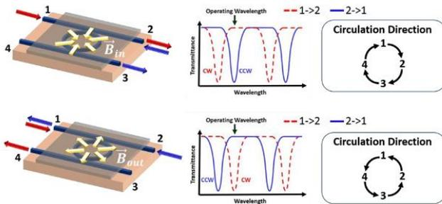
Figure 21. Integrated Isolator Design using Microring Resonator
