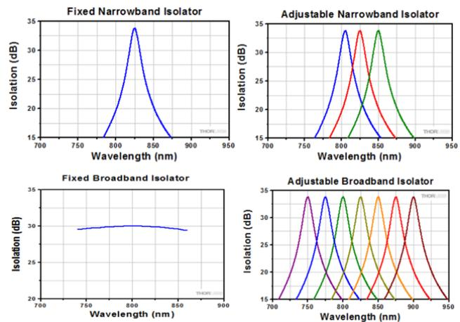
Figure 1. Broadband, Adjustable, and Narrowband Isolators from Thorlabs
