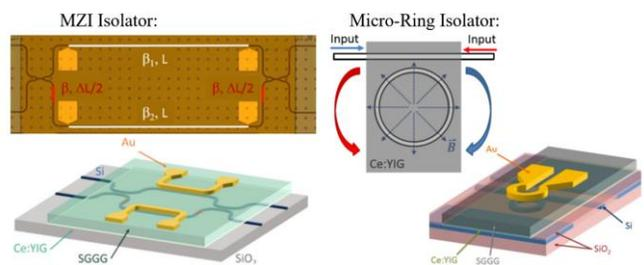
Figure 20. Integrated MZI and Micro-ring Isolator
