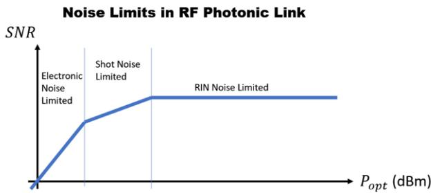
Figure 13. Noise Limits in an RF Photonic Link
