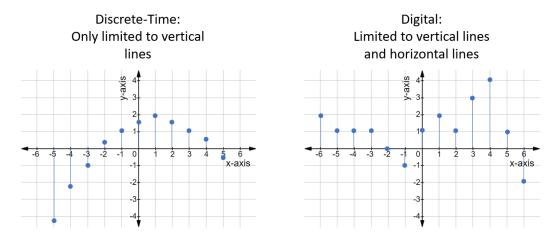
Discrete-Time Systems and Digital Systems are defined by their inputs and outputs being both either Discrete-Time Signals or Digital Signals.
